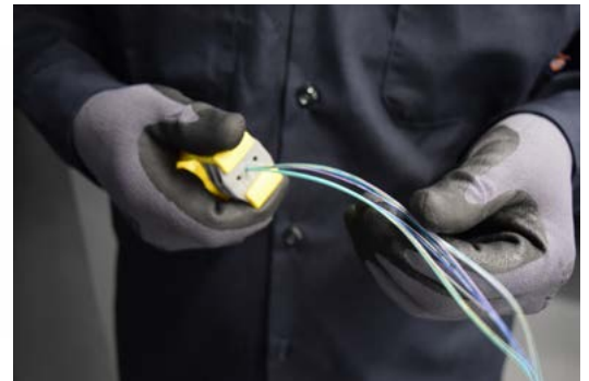
Release the tool and separate the cable elements
