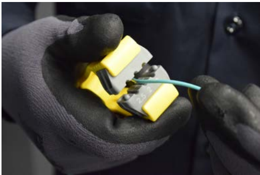
Align the fiber jacket or buffer tube to the proper channel
