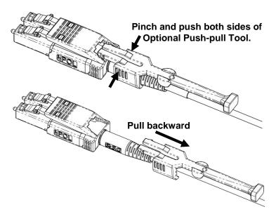
Pinch and push both front sides of Optional Push-pull Tool to warp inside. Keep warping inside and pull Optional Push-pull Tool backward to remove from connector.
