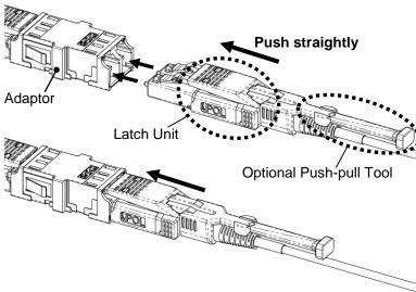
Hold Latch Unit or Optional Push-pull Tool, and push it straightly to the adaptor until clicking.
