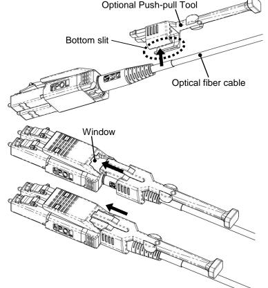
Put the optical fiber cable into the bottom slit of Optional Push-pull Tool.
